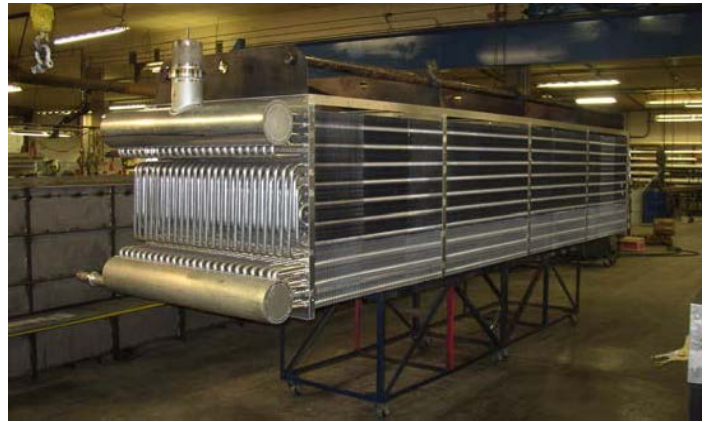
Figure 6 Al/Al Evaporator with Colmac BiM Connections
