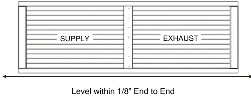
8.5.5. The heat pipe coil is manufactured with a dividing partition and frame such that standard duct flanges can be screwed to the frame. Use 3/16" diameter by 3/8" long self tapping sheet metal screws. Space as required. Do not allow drill bit to penetrate over 1/2" into the coil end boxes. Use of gaskets or sealants on the flange faces is recommended.
