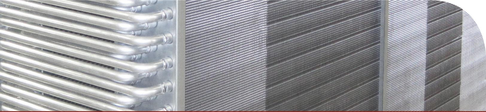
Colmac Coil heat pipe coils are designed to efficiently transfer heat from a warm air stream to a colder one. Heat pipes are constructed of a hollow tube lined with a capillary structure called a wick and a volatile refrigerant. When exposed to heat, the volatile refrigerant in the tube cycles endlessly between evaporation and condensation, effectively transferring the heat. This system has been proven to be at least 100 times more efficient in transferring heat than any solid conductor.
