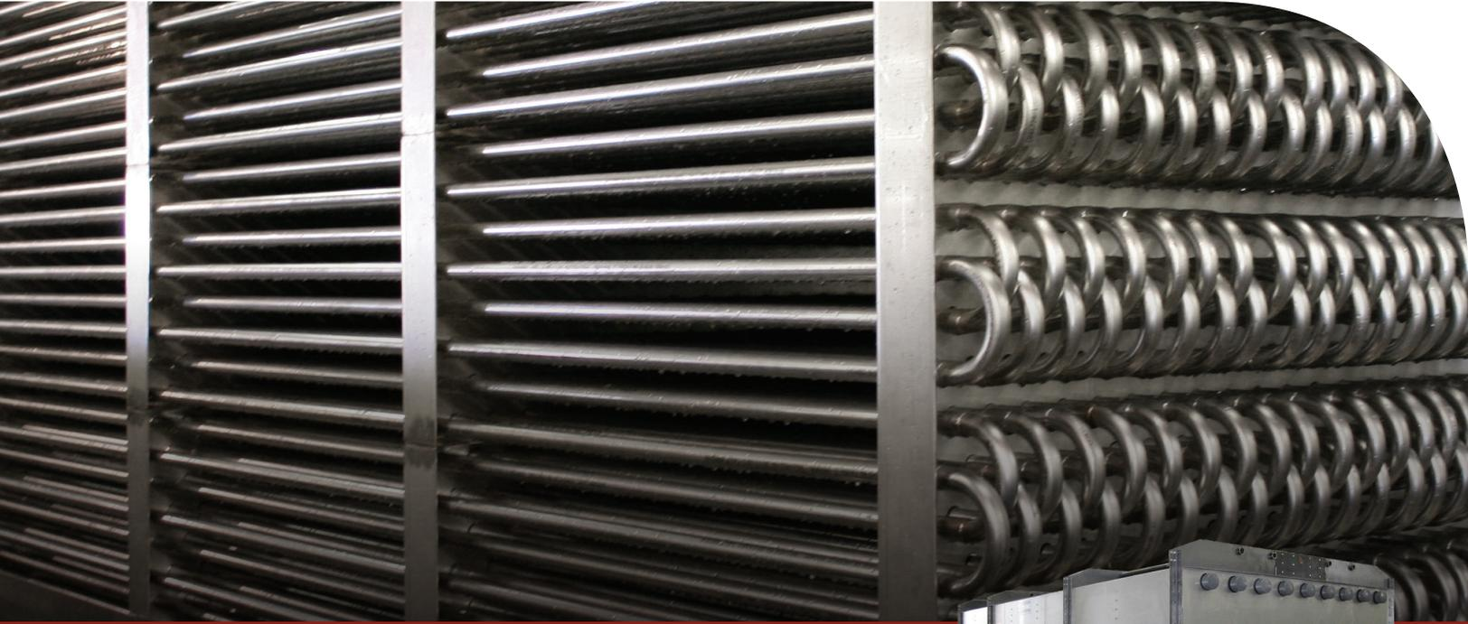
Hydrocoolers (also called Baudelot Coolers) are used in industrial applications for chilling a liquid to near its freezing point. Normally these coolers are used in systems where water is the liquid being chilled. A typical application is chilling process water used to take field heat out of agricultural produce.
